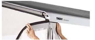
Front panels: slide into the awning's lead rail.
